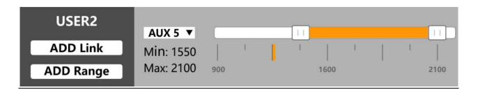
To activate or deactivate functions on the camera, you need to move the switch from the inactive state (white area) to the active state (yellow area), and then back to the inactive state (white area). To
