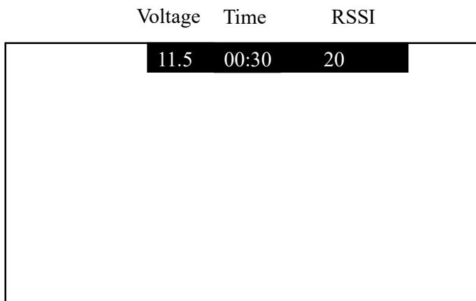
**Voltage indicator:** input voltage value is displayed; Display from 10V to 26 V. When the battery is low, the menu turns red and starts flashing. When the battery is too low, the blue light flashes faster and faster in the lower left corner and the buzzer alarms. Please replace the battery immediately to avoid damage to the battery.
